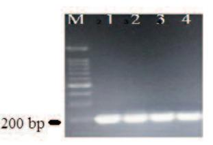
Figure 1. Gel electrophoresis of PCR product of *T. gondii* from buffy coat samples. Lane M: 100 bp ladder DNA size marker; Lane1: positive control; Lane 2–4: positive samples
