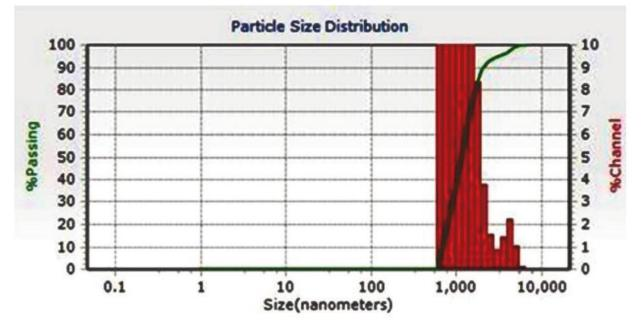
Figure 4. Particle size distribution of albendazole-nanocrystals using Dynamic Light Scattering (DLS)
