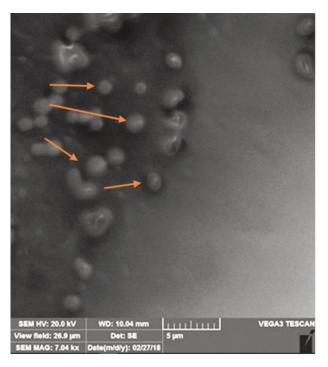
Figure 3. The SEM images of albendazole-nanocrystals. Nano-particles are shown with arrows. Scale bar is 5  $\mu$ m.
