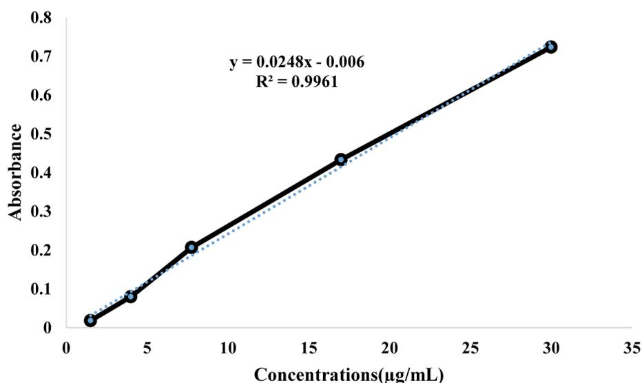
Figure 2. Standard curve of berberine chloride in 2- propanol solvent
